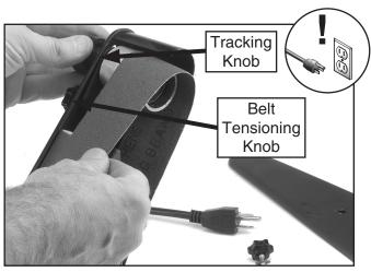
Figure 9. Installing belt.
